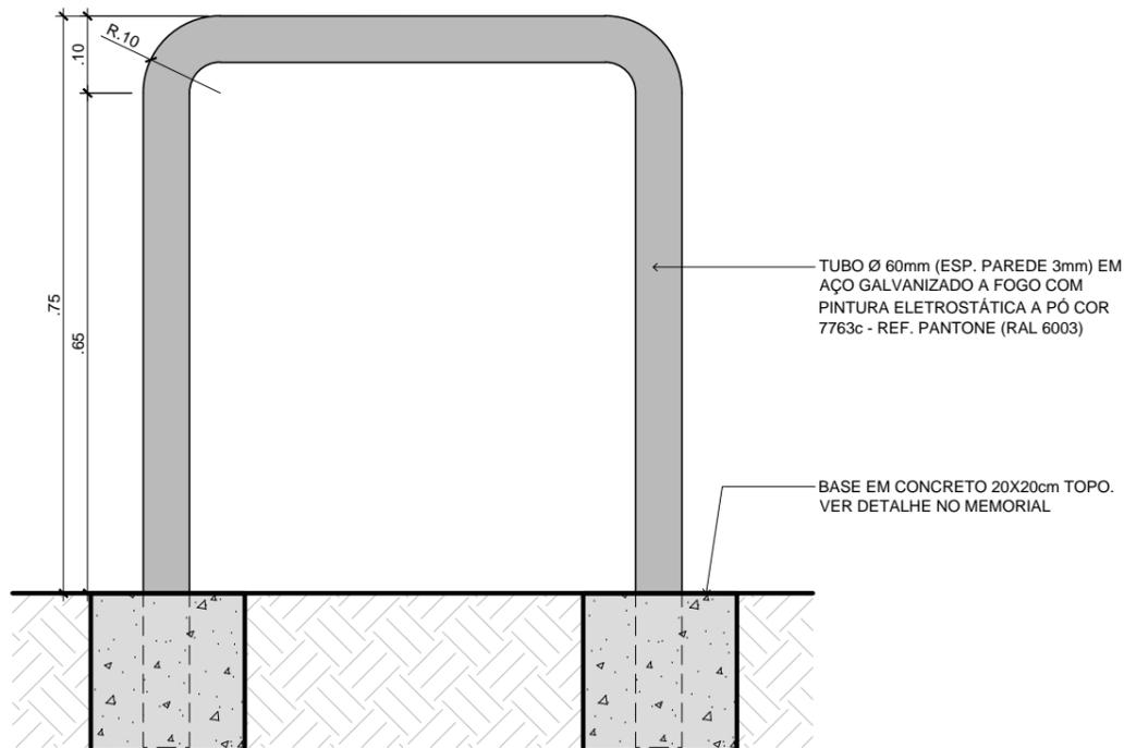
TUBO Ø 60mm (ESP. PAREDE 3mm) EM
