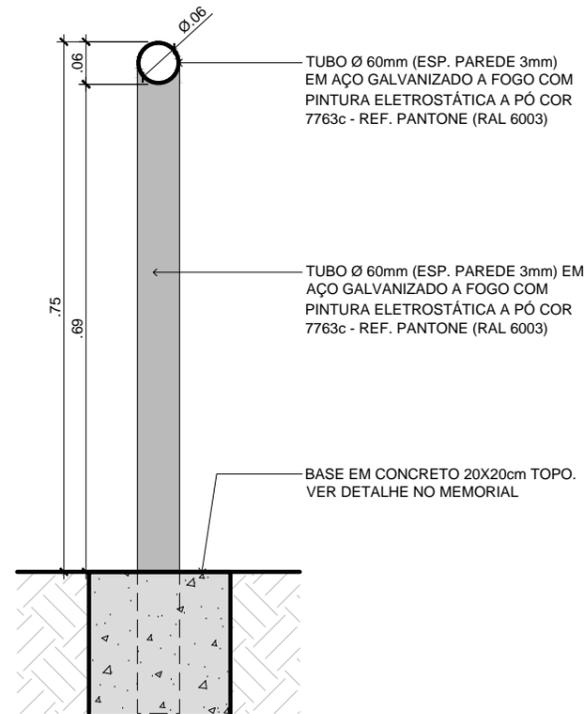
TUBO Ø 60mm (ESP. PAREDE 3mm)
