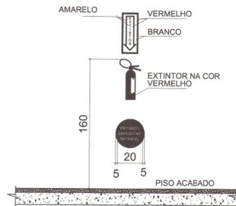
DETALHE DO EXTINTOR NA PAREDE
