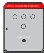
**DETALHE PAINEL DA BOMBA DE INCÊNDIO SEM ESCALA**
